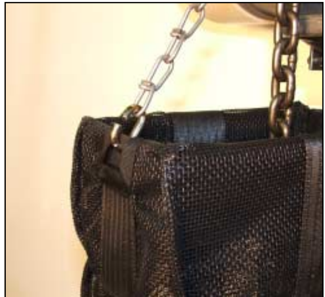
Figure 2. Support Chain Connection at Container
